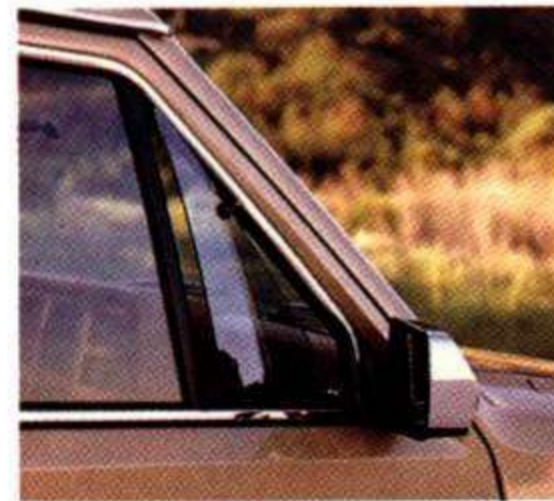
Optional swing-out vent windows allow additional flow-through of air.
