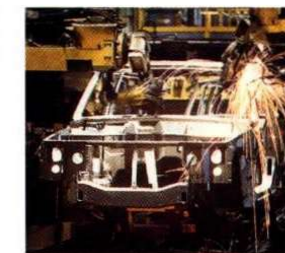
Comanche's unique UniFrame construction provides a lightweight yet rigid platform.
