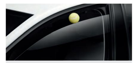
Anti-pinch protection windows protect you in case your arm is resting along the seam and the windows happen to shut. An important safety technology that prevents windows from closing, even when there is the slightest resistance or hand movement.
