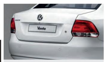
The Vento not only keeps you safe as you drive but also as you park. The rear parking sensors assist in parking manoeuvres by emitting audible signals. alerting the driver to any obstacles behind: the closer you are to an obstacle, the faster the sound frequency.
