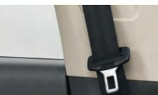
3-point seat belts are the primary means of protection and are available for front and rear outboard seat occupants. The front seat belts are height-adjustable for a more comfortable and secure fit.
