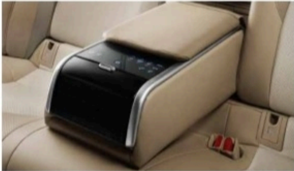
REAR ARMREST WITH CAPACITIVE TOUCH-CONTROL SWITCHES FOR AUDIO, REAR RECLINE, REAR SUNSHADE AND AC CONTROL
