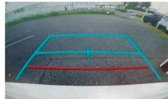
PARK ASSIST: BACK MONITOR WITH DYNAMIC GUIDELINES & CLEARANCE SONAR
