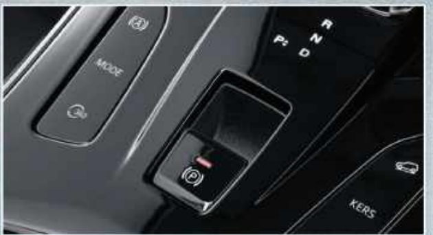
THE ELECTRIC PARKING BRAKE (EPB) AND AUTO VEHICLE HOLD (AVH) PREVENT THE VEHICLE FROM ROLLING WITHOUT THE NEED TO CONTINUOUSLY PRESS THE BRAKE.
