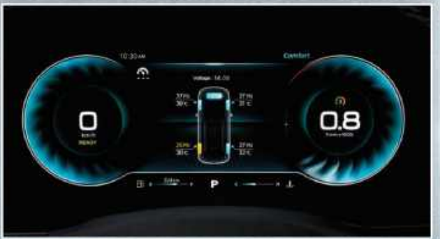
THE TPMS IS DESIGNED TO MONITOR FOR ANY ABNORMALITIES IN TIRE PRESSURE, ENHANCING SAFETY.
