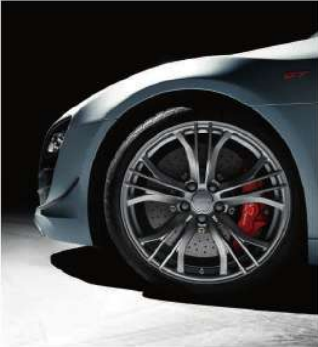
■ Forged aluminium wheels in 5 double-spoke Y design in titanium look, size 8.5 J x 19 at front, size 11 J x 19 at rear, with 235/35 R 19 tyres at front and 295/30 R 19 tyres at rear S
