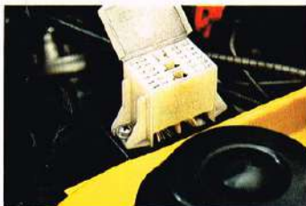
This plug will connect your Audi 80 with the AUDI NSU Computer Diagnosis System.
