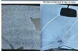
Laminated safety windshield (right)
