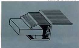
Bonded windshield & rear window
