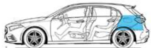
Open luggage compartment behind rear seat, loaded to upper edge of rear seat backrest, volume 355 litres (V 211-2)
