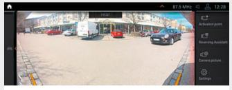
☐ The Crossing traffic warning\* rear warns you of crossing traffic when pulling out of perpendicular parking spaces. The system works up to a speed of 7 km/h and can be activated and deactivated via the "Park" setting menu.
