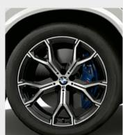
21" M light alloy wheels Y-spoke style 741 M Bicolour Orbit Grey with mixed tyres, burnished, front 9.5J x 21 with 275/40 R21 tyres, rear 10.5J x 21 with 315/35 R21 tyres<sup>2, \*</sup>.
