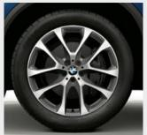
☐ 20" light alloy wheels V-spoke style 738 in Bicolour with mixed tyres and runflat properties. burnished, front 9J x 20 with 275/45 R20 tyres, rear 10.5J x 20 with 305/40 R20 tyres.2
