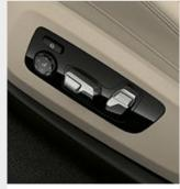
☐ The lumbar support for the driver and front passenger seats can be adjusted both vertically and laterally, allowing for an orthopaedically optimised seating position.
