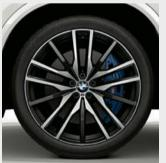
$\square$  22" M light alloy wheels Double-spoke style 742 M Jet Black with mixed tyres, front 9.5J x 22 with 275/35 R22 tyres, rear 10.5J x 22 with 315/30 R22 tyres.
