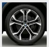
☐ 21" light alloy wheels Y-spoke style 744 Bicolour Orbit Grey with mixed tyres and runflat tyres, burnished, front 9.5J x 21 with 275/40 R21 tyres, rear 10.5J x 21 with 315/35 R21 tyres.<sup>1,5</sup>
