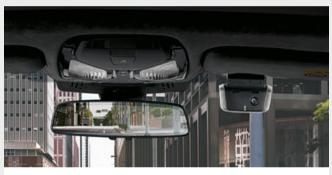
O The BMW Advanced Car Eye 2.0 is a highly sensitive full-HD camera that captures events in front of and behind the car, even when it is parked. In the event of disturbances and extraordinary movement outside the vehicle, the camera automatically records the situation in order to document possible accidents or (attempted) break-ins.
