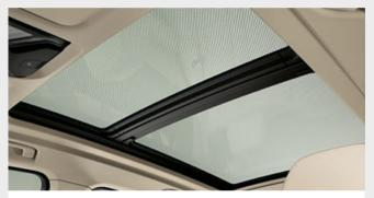
☐ When open, the Panorama glass roof provides a great deal of fresh air. Closed, it creates a bright, light-flooded atmosphere in the interior. It opens and closes completely automatically at the push of a button, or remotely, and is equipped with slide and lift functions, roller sunblind and wind deflector.
