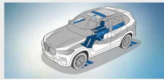
☐ Active Protection is a preventive occupant protection system that pretensions the seat belts in critical situations, puts electric seats in an upright position and closes windows and the sunroof, if featured.
