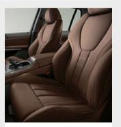
☐ The seat heating increases the temperature of the seat and backrest surfaces of the front seats as well as the exterior rear seats. It can be individually regulated to three levels for each seat.
