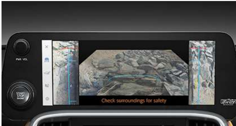
Underfloor View & Both-sides View
