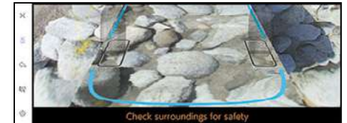
Underfloor View (Rear wheels) (Enlarged)
