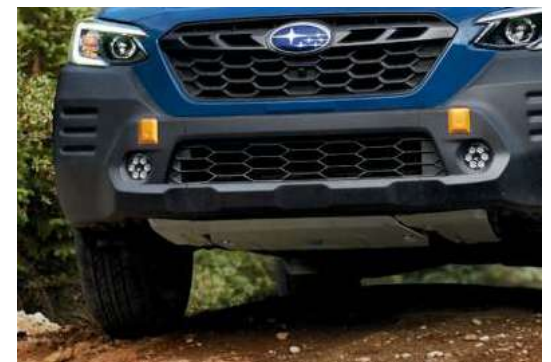
Protective under-body skid plates: front lower, engine, transmission and rear differential
