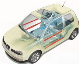
The bodywork is more resilient, featuring double side-impact bars.
