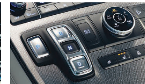
Shift-by-Wire push-button gear selection
