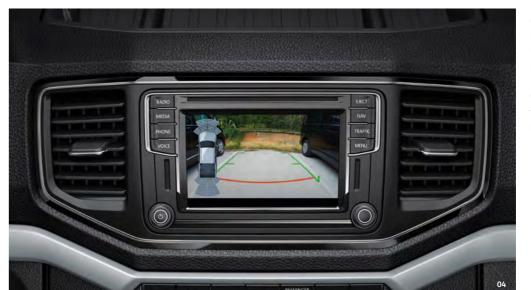
**04 "Rear View" reversing camera** simplifies parking by showing a limited view of the area behind the vehicle on the display. Static guidelines facilitate the parking process.
