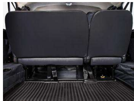
For transportation of large-size cargo and equipment the rear seats can be folded down 60/40 or turned into a bed by extending to 180°
