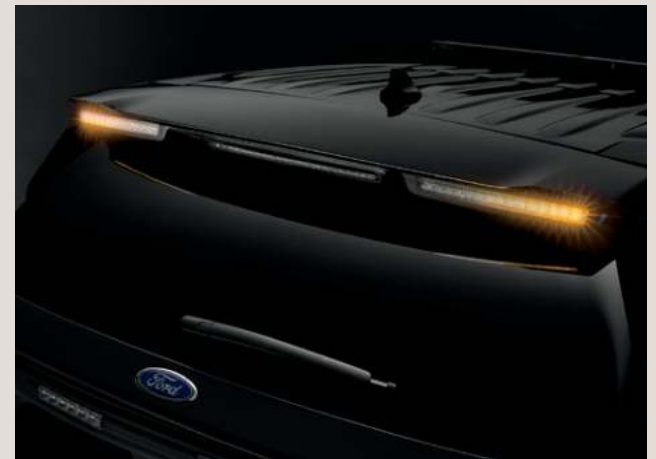
Rear spoiler LED traffic warning lights (96T). Includes (2) backlit flashing, linear high-intensity LED lights (driver side red; passenger side blue) mounted on the edge of the rear spoiler. Lights can be programmed for tricolor (red, blue, amber) patterns; also features amber-only traffic direction mode.
