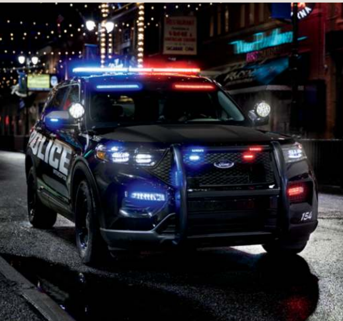
Front Headlamp Lighting Solution (66A). Includes base headlamps with LED high- and low-beam wig-wag function and LED side warning lights (driver side red/white; passenger side blue/white).
