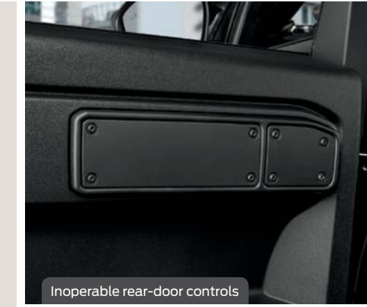
Inoperable rear-door controls
