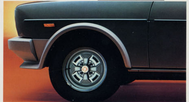
Wheelarch mouldings of sports design, connected with the bumpers and the door sills. Functional body protection against stone chipping.
