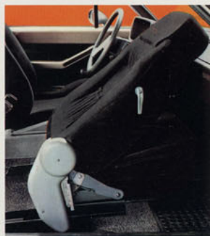
Folding front seatbacks with simultaneous forward travel of the seats. Easy access to the rear seats.
