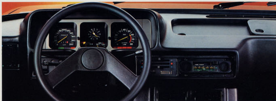
Dashboard made from energy-absorbing material. Comprehensive instrumentation. Glove box with two sliding lids. Two-spoke steering wheel covered in padded non-slip material. Safety and sportiness.
