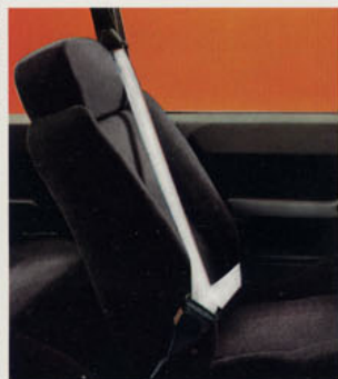
Inertia reel, three-point attachment seat belts. Comfort and safety.
