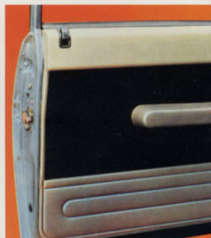
Air extractors on door panels. Demisting of side windows.
