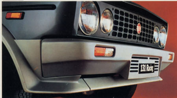
Front spoiler connected with the bumpers. Increased tyre adhesion at high speed and reduced aerodynamic drag.
