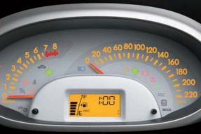
Distinctive double meters are positioned on the steering column close to the driver for visibility suited to driver physique Illustrated meters are for 1.3-litre engine models.
