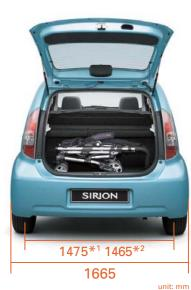
\*1: Models equipped with 13-inch wheels \*2: Models equipped with 14-inch wheels
