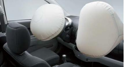
Front SRS air bags for driver and front passenger help to prevent occupant injuries in the event of a collision.
