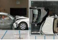
SIRION's impact-absorbing body Extensive crash testing was conducted structure reduces deformation in a in pursuit of a high level of occupant safetv.
