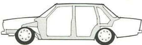
The Volvo body is designed so that the passenger compartment will stay intact even under severe impact conditions.
