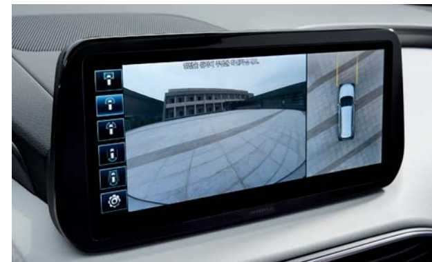
Blind-spot View Monitor Engaging the turn signal in either direction shows the driver video footage of what's next to and behind the car in the instrument cluster.
