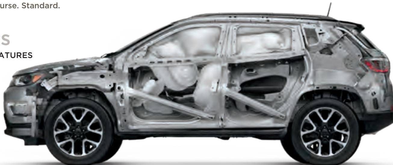
**A Secure Air Bag<sup>8</sup> System** Your need for security is fully respected with this all-around air bag<sup>8</sup> system. Full-length side-curtain, seat-mounted side thorax, and advanced multistage front and driver's inflatable knee bolster air bags<sup>8</sup> all work together to help provide protection. Standard.
