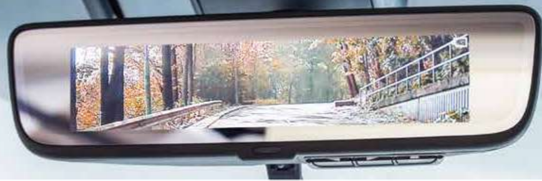
電子影像倒後鏡，清晰顯示車後路面情況 Digital Inner Rear-view Mirror shows the road conditions behind the vehicle
