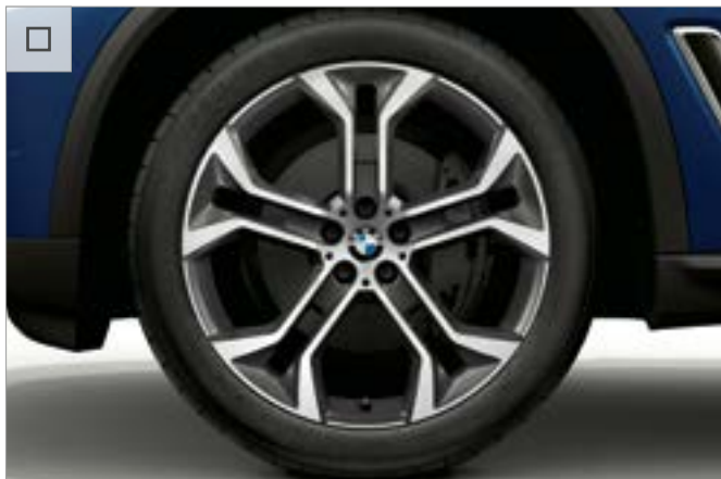
21" light alloy Y-spoke style 744 wheels, Bicolour, front 9.5 J x 21 with 275/40 R21 tyres, rear 10.5 J x 21 with 315/35 R21 run-flat tyres. (Optional for xLine models only).
