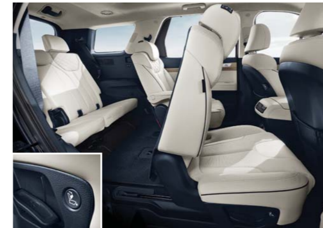
Smart, one-touch, second-row folding and sliding seats When you push the walk-in button installed on the sides of the second-row seats, the seats fold down and slide back, making it easy to access the third row.
