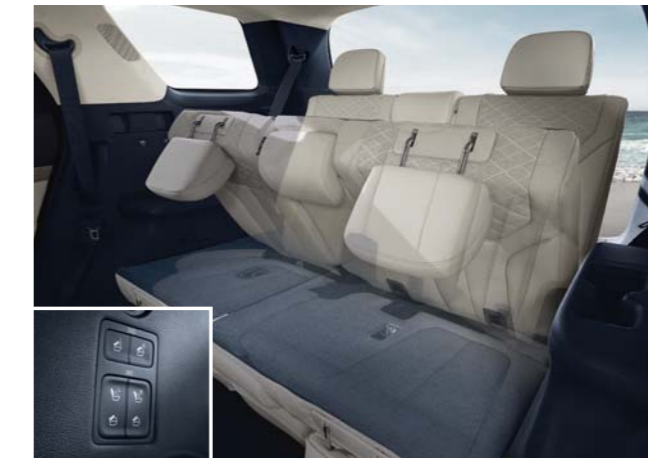
Third-row power folding seats / Second-row smart one touch folding At the push of a button, you can fold away or unfold the third-row seats as well as control the second-row seats to provide easier access to the third-row seats or increase cargo space.
