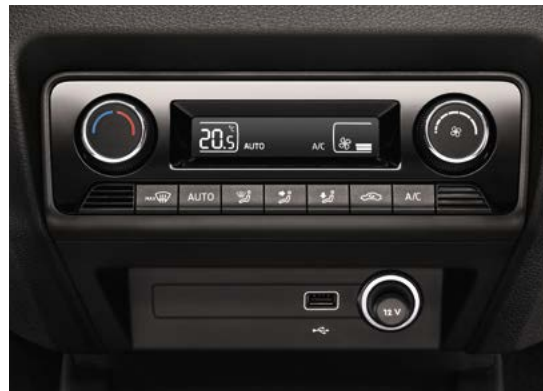
CLIMATE CONTROL AIR CONDITIONING
