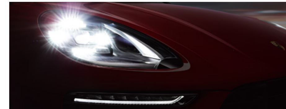
Main beam with LED main headlights
