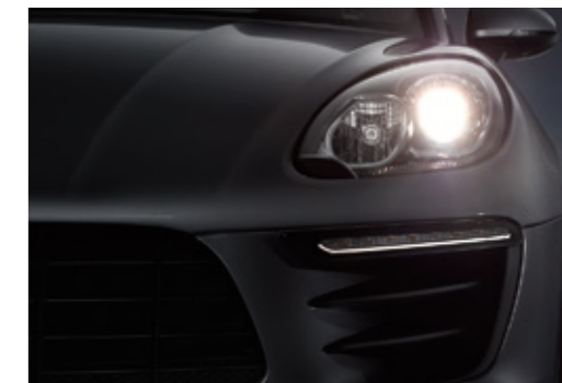
Dipped beam with halogen headlights
