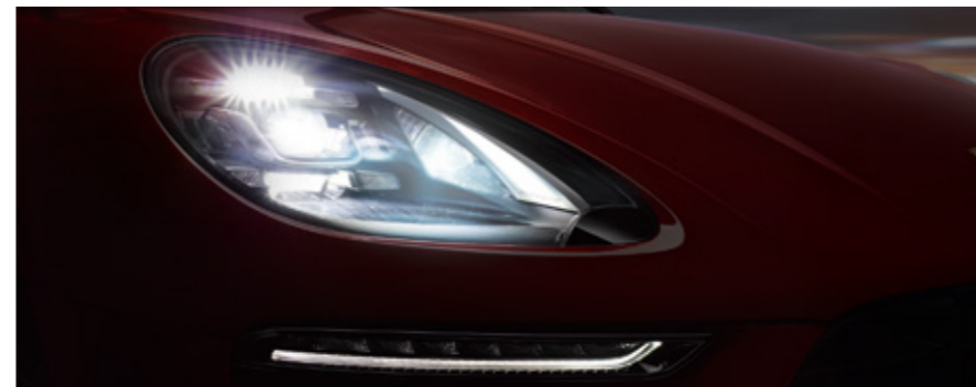
Dipped beam and cornering lights with LED main headlights
