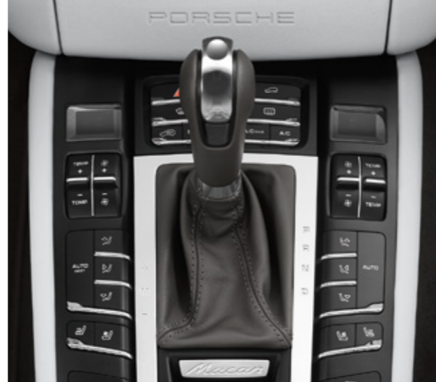
Climate control buttons in front for three-zone automatic climate control
