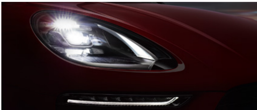
Dipped beam with LED main headlights
