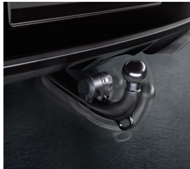
Electrically extending towbar system
