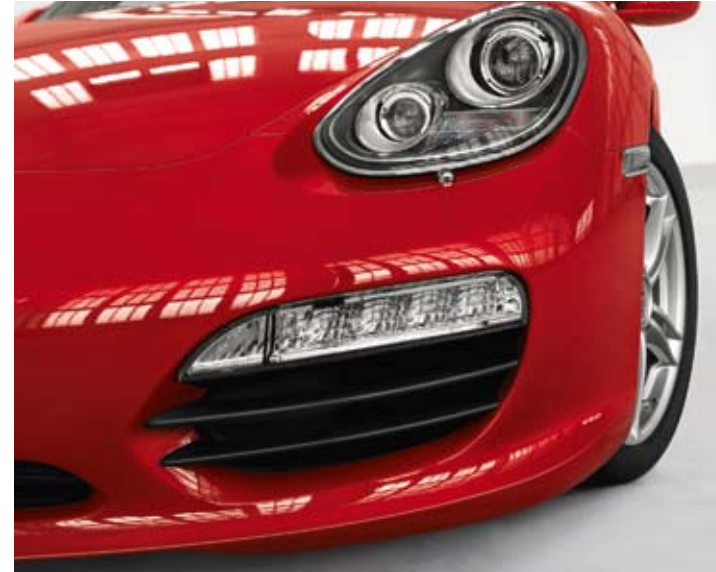
Air intake grilles
