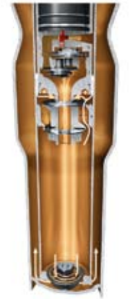
Compression in 'Normal' mode – working piston and bypass, sporty-hard tuning
