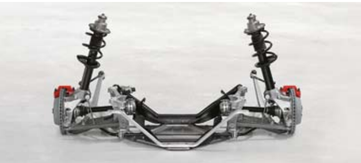
Rear axle with McPherson struts and lateral control arms (Boxster S)
