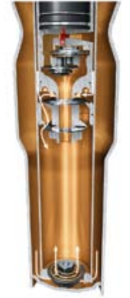
Rebound in 'Sport' mode – working piston only, sporty-hard tuning
