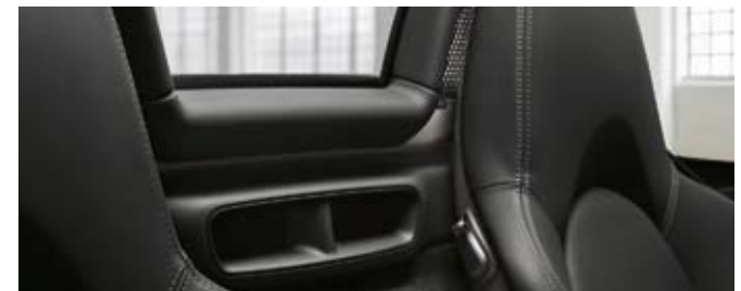
Active subwoofer with 2 x 13 cm low-range speakers and 2 x 6.5 cm mid/high-range speakers
