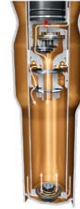
Rebound in 'Sport' mode – working piston only, sporty-comfortable tuning
