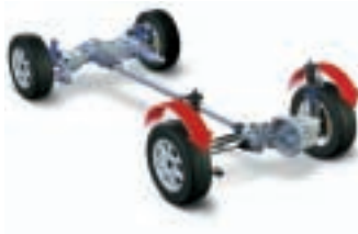
If you are cruising on straight, dry roads, the car is almost entirely front-wheel driven for optimum stability and fuel economy.
