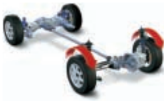
When braking, the car disengages drive to the rear wheels the instant you touch the brake pedal, thereby maximizing control and roadholding.
