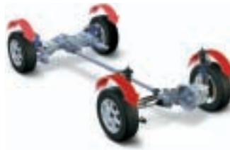
If the front wheels show any tendency to spin, the AWD system responds instantly by redistributing up to 50% of the power to the rear wheels for maximum traction and stability.
