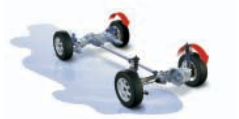
If one or both wheels on one side of the car spin, more power goes instantly to the wheels on the opposite side with the best traction.
