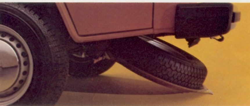
Up-front, under-floor spare tire storage—more room inside.
