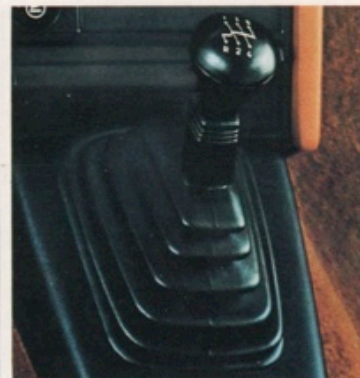
Available 5-speed manual transmission
