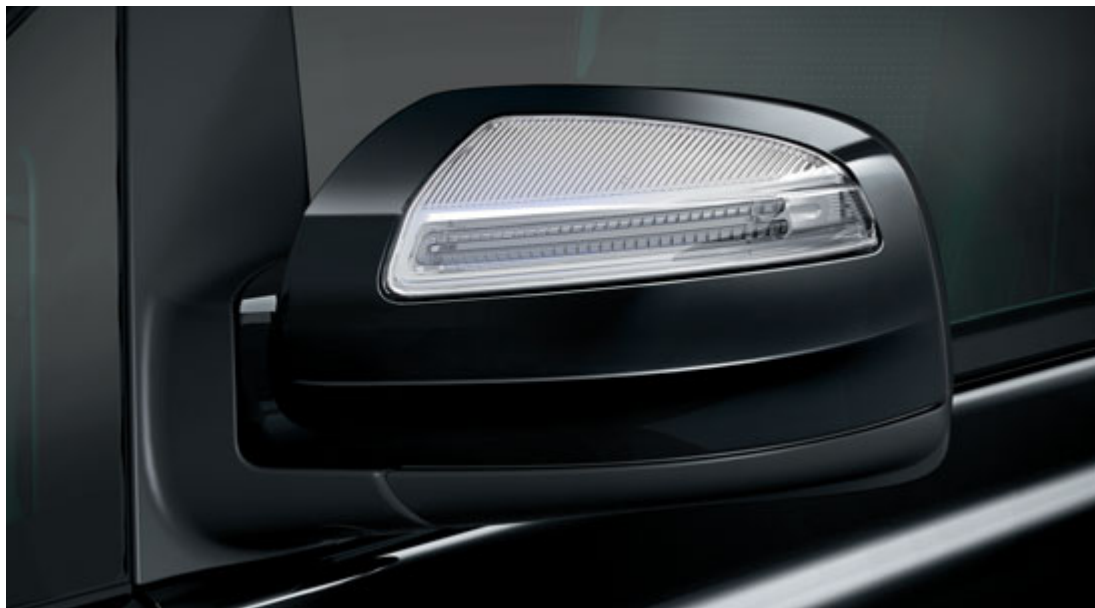
Exterior mirrors with greater field of vision and integral indicator lamp, electrically adjustable
