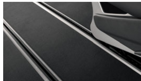
The seat rail system for variable configuration of the interior
