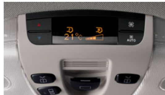
Additional heat exchanger for the rear with separate control unit
