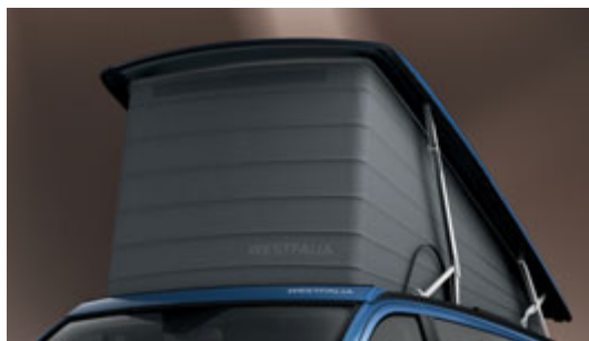
EASY UP electrohydraulic pop-up roof
