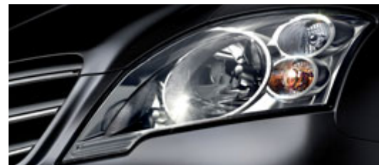
Refl. headlamps: fr. fog lamps & daytime driving lights
