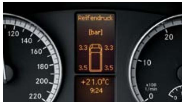
The automatic tyre pressure monitoring system
