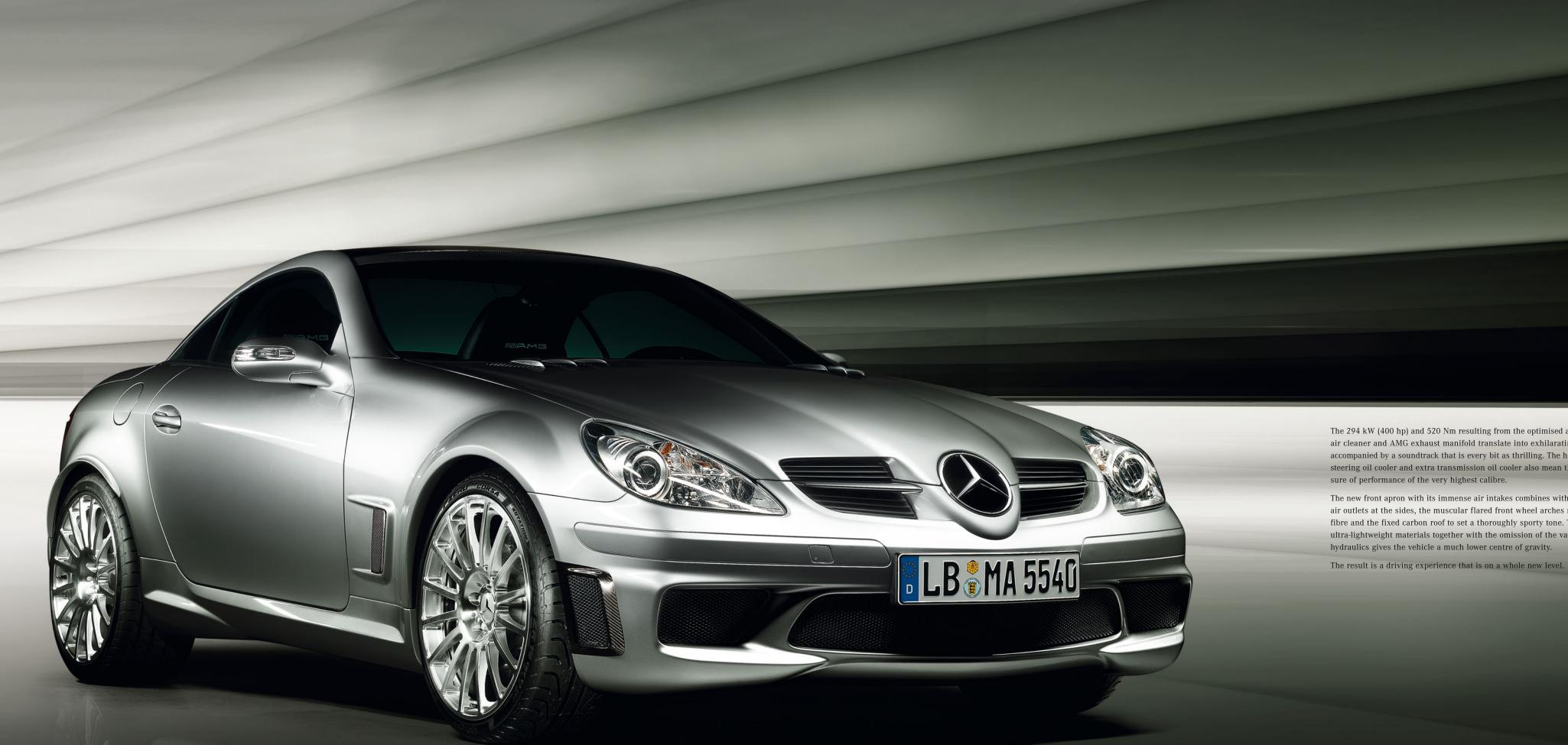
The 294 kW (400 hp) and 520 Nm resulting from the optimised air intake, sports air cleaner and AMG exhaust manifold translate into exhilarating propulsion accompanied by a soundtrack that is every bit as thrilling. The high-performance steering oil cooler and extra transmission oil cooler also mean that you can be
