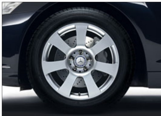
7-spoke light-alloy wheel with 235/55 R 17 tyres (standard for V6 engines)
