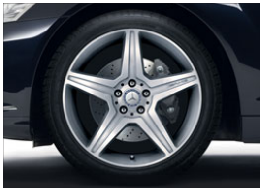
AMG 5-spoke light-alloy wheel with 255/40 R 19 front and 275/40 R 19 rear tyres (AMG Sports package)
