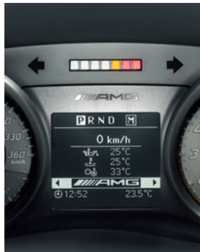
AMG instrument cluster with 7-LED upshift indicator
