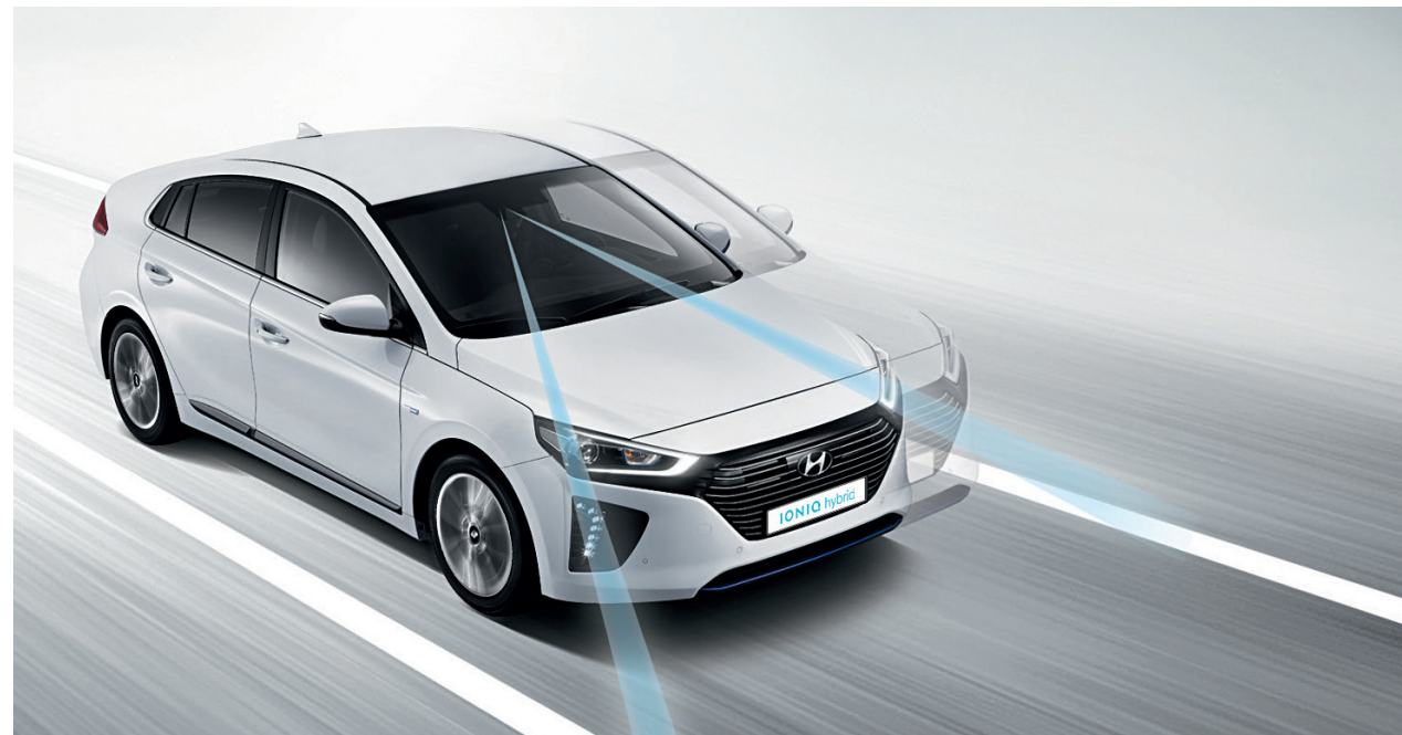
Lane Departure Warning System with Lane Keep Assist (LKAS)*
