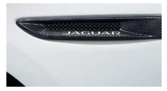
Carbon Fibre Side Power Vent T4A12419 - Left Side T4A12418 - Right Side
