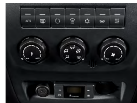
HVAC control panel
