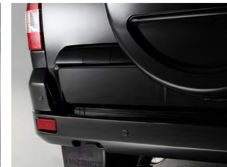
Body coloured rear bumper with integrated parking sensors
