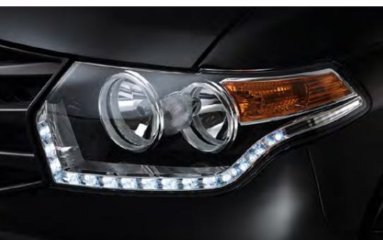
Headlamps with LED daytime running lights
