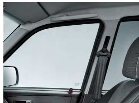
Height-adjustable seat belts
