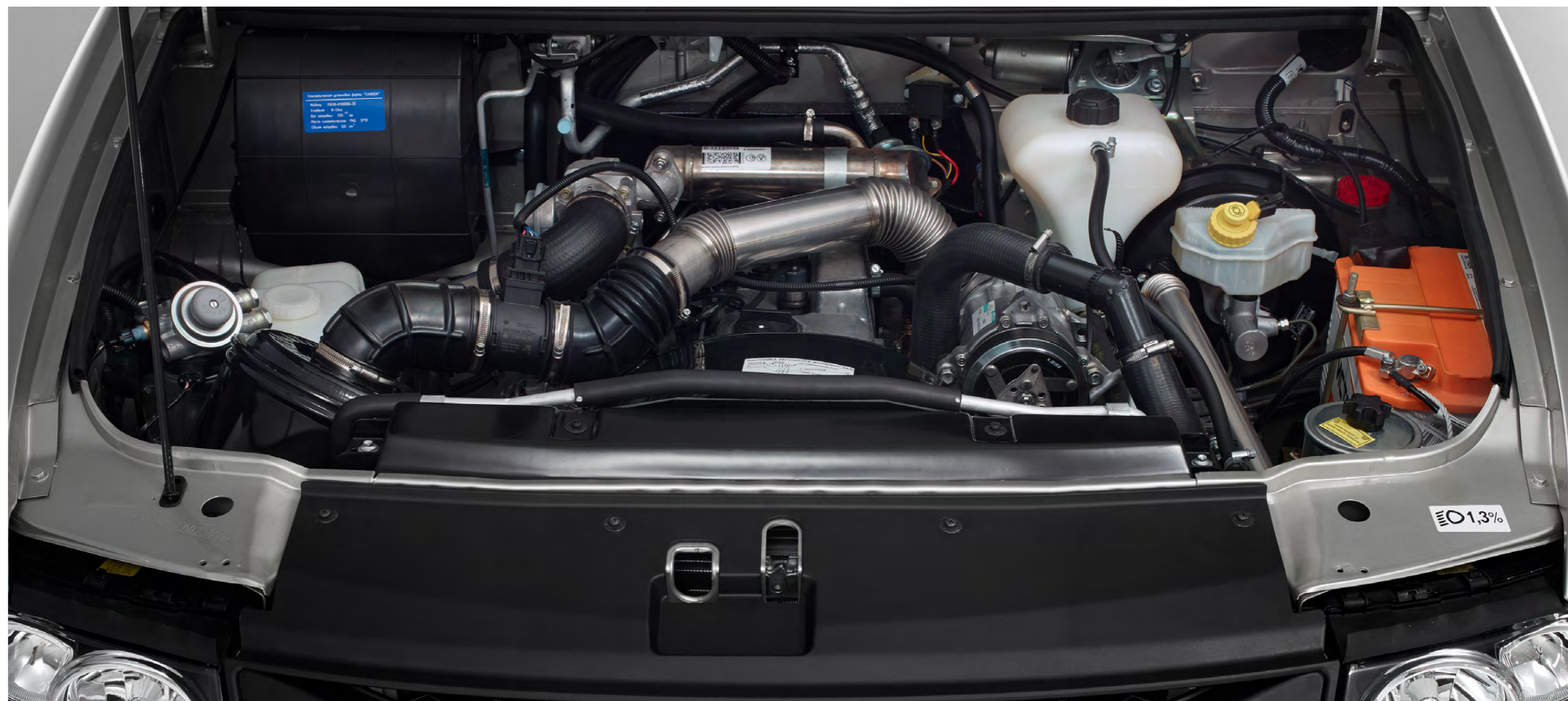
Diesel engine with 2.2 L displacement, 114 hp
