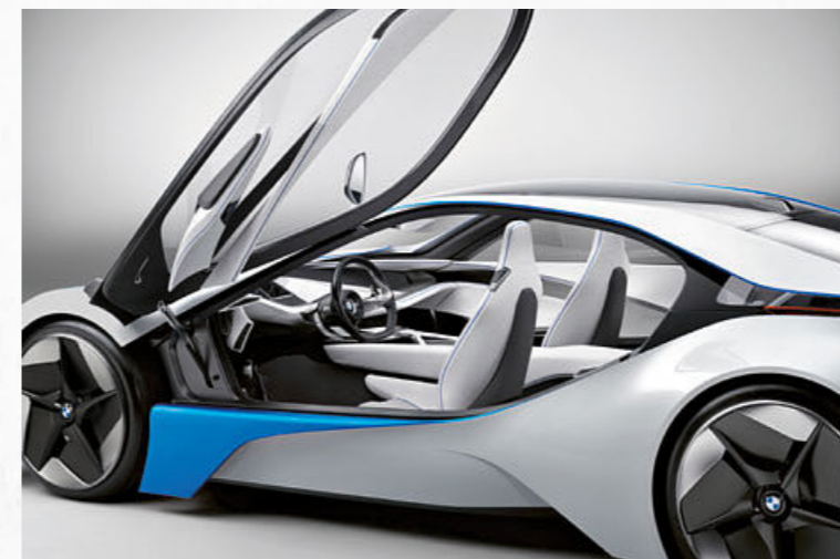
The distinctive dihedral doors were already a visual highlight in the BMW Vision EfficientDynamics concept vehicle.
