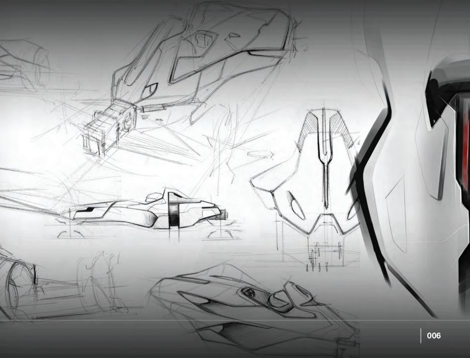
While this futuristic vision runs throughout Mono's appearance it was fundamental to our designers that form follow function on all aspects of the car. The necessity to gain access to the central driving position and adjustable dampers as well as providing clean airflow to the radiators and engine are just some of the factors on which Mono's architecture is built.
