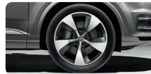
Forged aluminium wheels in 5-arm turbine, contrasting grey, partly polished 2 size 9.5 J x 21 with 285/40 R 21 tyres 1
