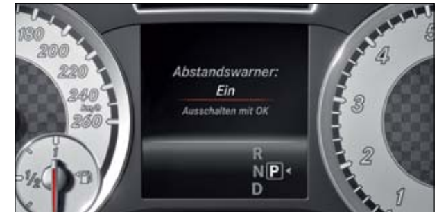
COLLISION PREVENTION ASSIST can recognise a safety distance that is too short and warn the driver.
