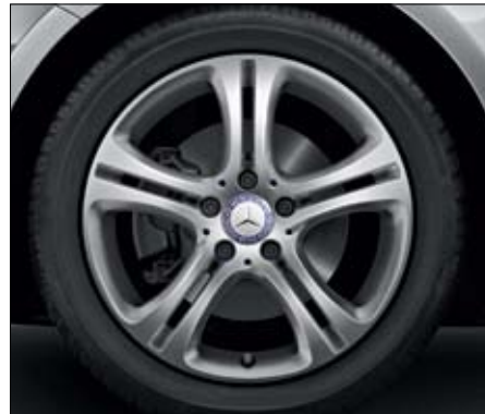
5-twin-spoke light-alloy wheels with 225/45 R 17 tyres (standard in conjunction with Urban, Code R11).
