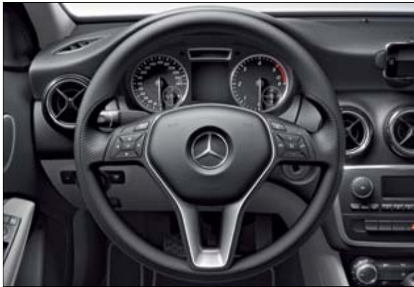
3-spoke multifunction steering wheel with 12 function buttons.
