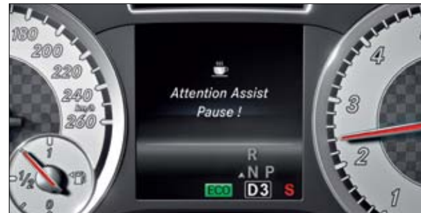
If ATTENTION ASSIST detects signs of driver drowsiness it recommends taking a break.
