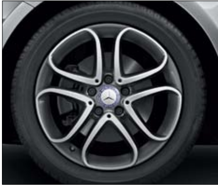
5-twin-spoke light-alloy wheels painted himalayas grey with a high-sheen finish, with 225/45 R 17 tyres (option, Code R48).
