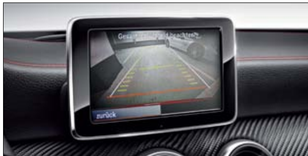
During parking, the COMAND Online central display shows the area behind the car.
