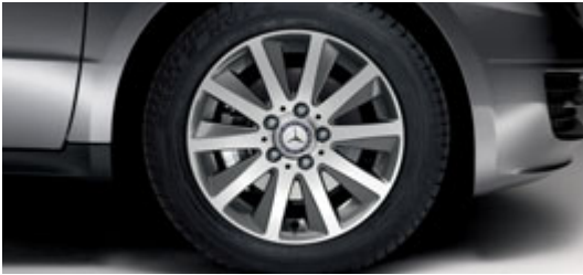
Bicolor light-alloy wheels in 10-spoke turbine design with 195/55 R 16 tyres (optional)
