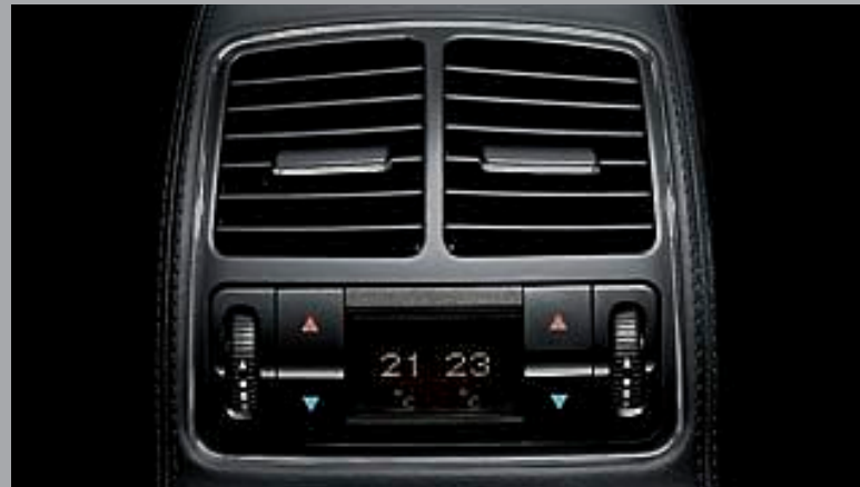
The THERMOTRONIC luxury automatic climate control system also allows the rear occupants to choose their own temperature settings
