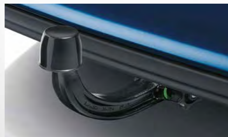
DETACHABLE TOW BAR HATCH - 52038944 • SEDAN - 52032403 TOW BAR WIRING HARNESS - 50927832
