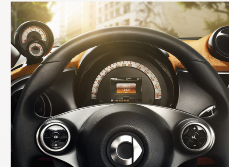
The instrument cluster with with a colour 8.9 cm (3.5-inch) TFT display 1 has all the data and information you need during your journey. As an option you can supplement the information centre of your smart fortwo with a dashboard instrument showing the revs and the time.
