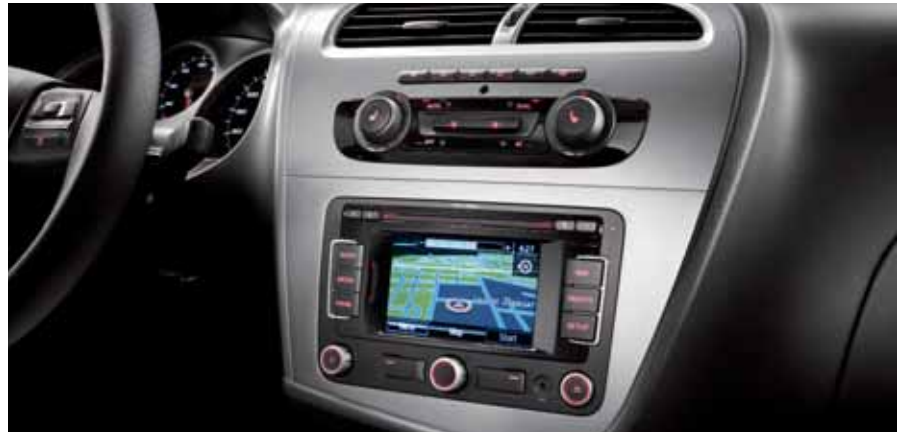
SEAT Media System 2.2 with Bluetooth®, touch screen and DAB (Digital Audio Broadcasting).
