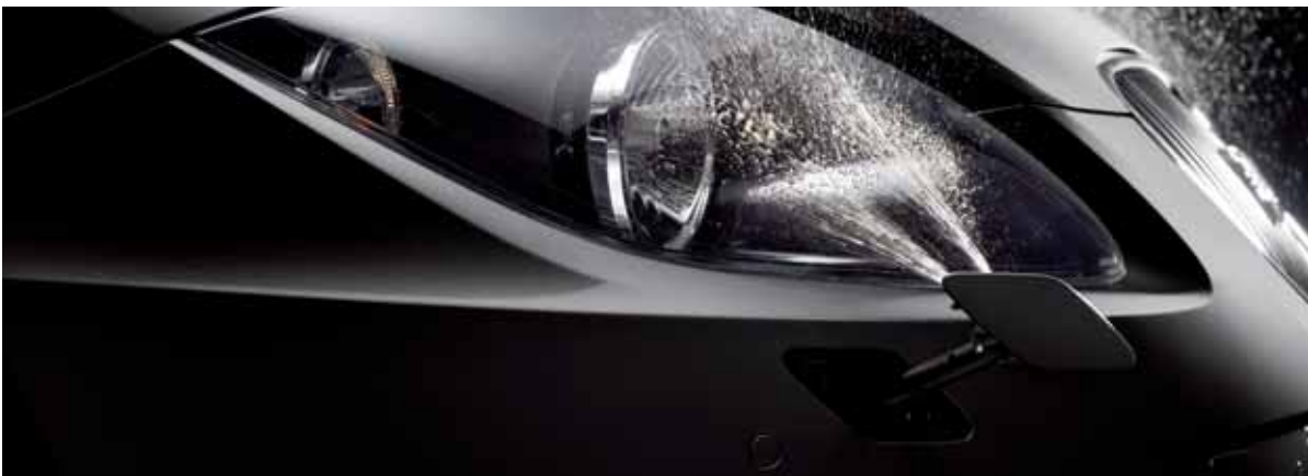
Headlight washer system (included with the bi-xenon headlights and in the Winter Pack).
