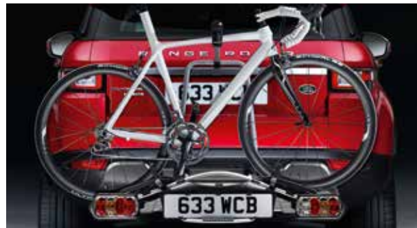
Tow Bar Mounted Bike Carrier* Δ VPLVR0066 – Two Bike Carrier VPLVR0068 – Three Bike Carrier The tow bar mounted bike carrier features a one hand, quick attach/release tow bar coupling mechanism and can be tilted away from the vehicle, by use of a foot pedal, to allow easy access into the rear tailgate. The tailgate can be opened with carrier in deployed/folded position. Manufactured from aluminium and other lightweight materials, the bike carrier also features a rear lighting and licence plate mount and it is lockable for security. The carrier has a folding/sliding mechanism to allow ease of stowage when not in use. A holder and ratchet function ensure bicycles are safely secured. Maximum load capacity 40kg.
