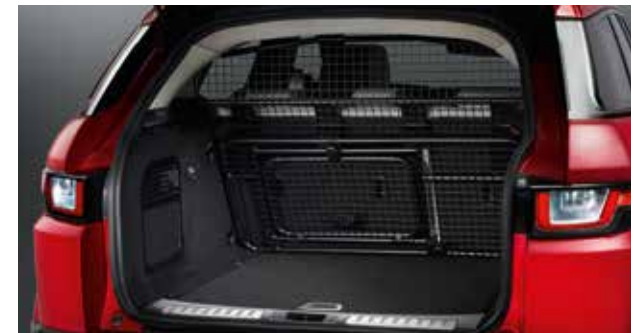
Luggage Partition Full Height* VPLVS0221 – Coupé VPLVS0220 – Five-door Designed to prevent luggage from entering the passenger compartment. Easily removed. Complies with ECE-17 regulation.
