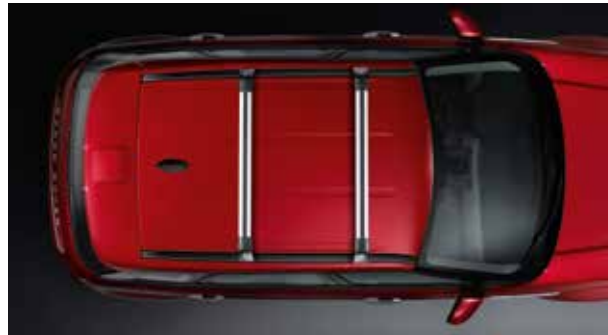
Cross Bars* Δ VPLVR0073 Silver finish, adjustable position cross bars for vehicles fitted with roof rails. Aerodynamic profile designed to minimise drag and noise. Lockable for security and incorporating a T-slot to carry the Land Rover roof mounted accessory range. Vehicle height when fitted: Coupé 1,697mm/Five-door 1,720mm. Maximum permissible load capacity 71.8kg.**
