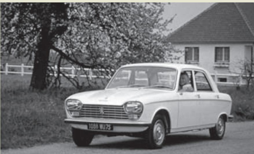
**1965 - 1966** Peugeot unveils its revolutionary 204, the first of its cars to feature front-wheel drive. It is powered by a light alloy engine with overhead camshaft and features four independent wheels and front disk brakes. The Société des Automobiles Peugeot becomes Peugeot S.A., a holding company controlling all the companies in the Group.
