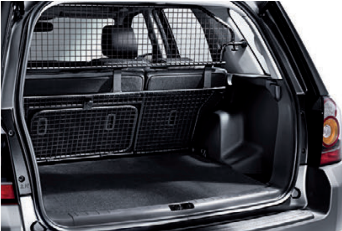
Cargo Barrier LR002521 Easily removed. Retains cargo according to EC Regulation 17.
