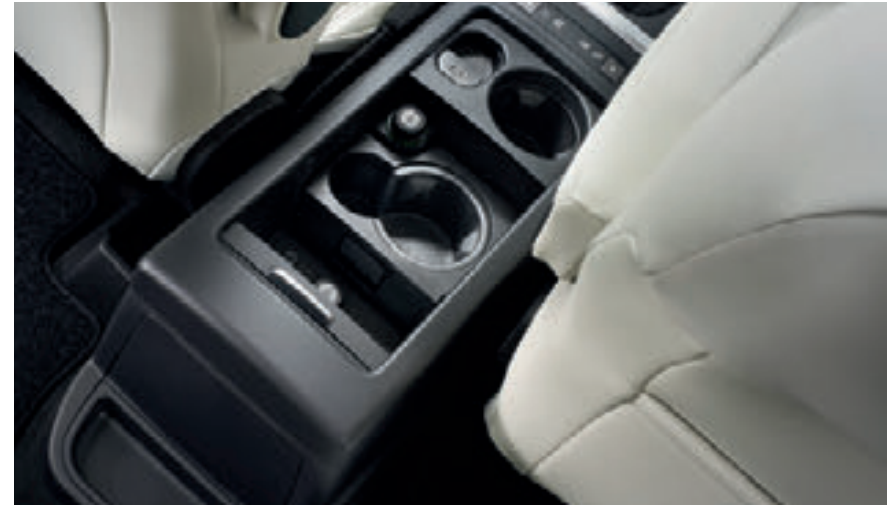
CENTRE CONSOLE STORAGE. The rear of the centre console features an additional storage box for small items, an audio socket for MP3 players and a power socket, which can be used to recharge PCs and other low-wattage electrical equipment.
