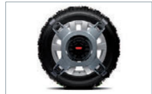
Snow Traction System LR005169 For 17 inch and 18 inch front wheels only.
