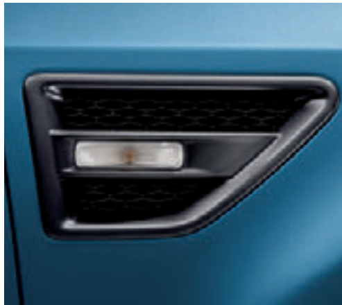
Side fender vents in Brunel
