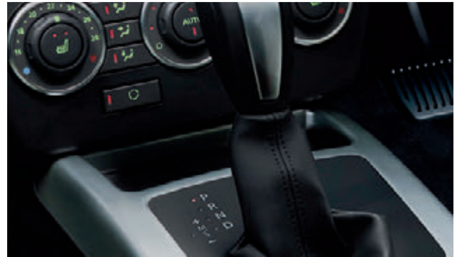
COMMANDSHIFT®. The six-speed automatic transmission with CommandShift is standard on SD4 diesel models and optional on TD4 diesel models. CommandShift® provides manual sequential gear changes and Sport mode for an even livelier performance. (Not available on eD4).
