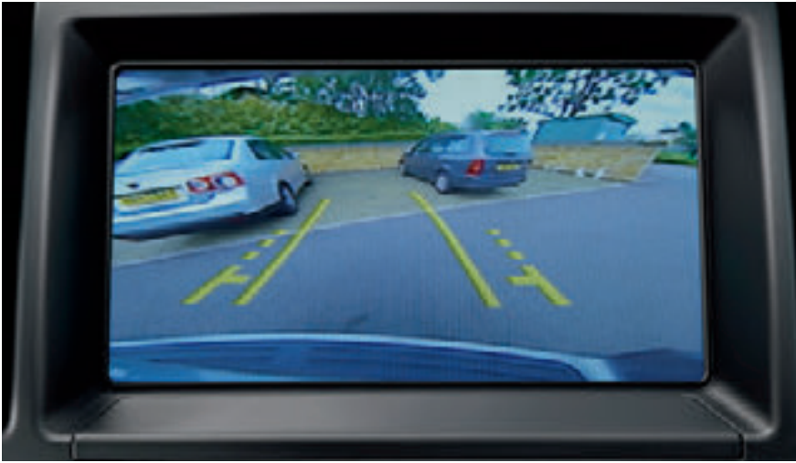
REAR VIEW CAMERA. The Rear View Camera helps reversing by displaying a wide-angled rearward view from the vehicle on the centre console screen. To aid manoeuvrability, lines representing the vehicle's predicted path are superimposed on the image. Includes trailer hitch assist.
